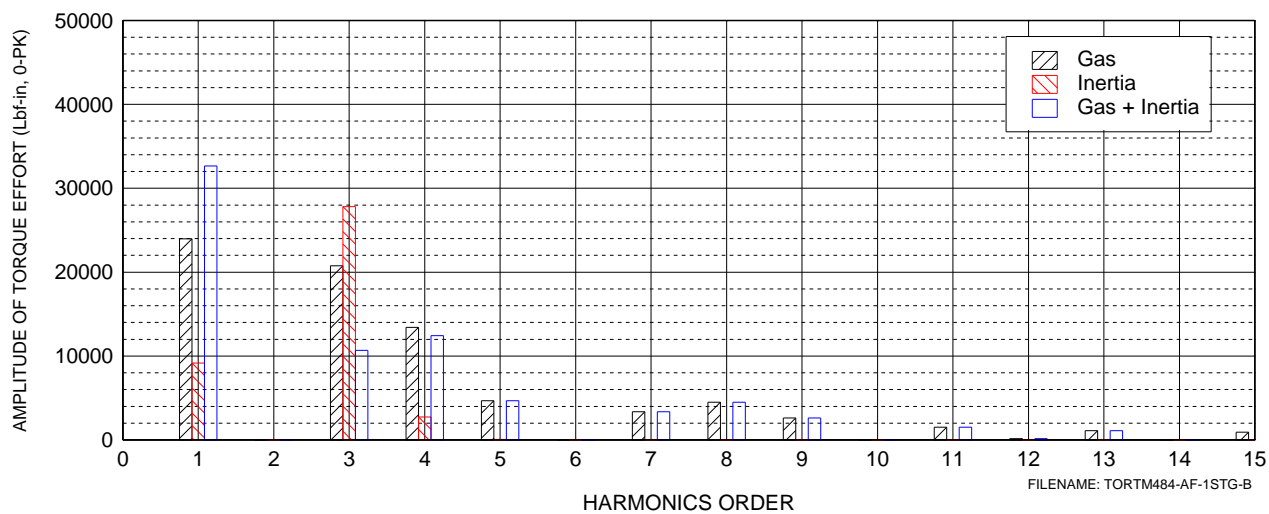
Figure 3.1: One stage torque effort - approximately 4200 lb r -in at 5x
