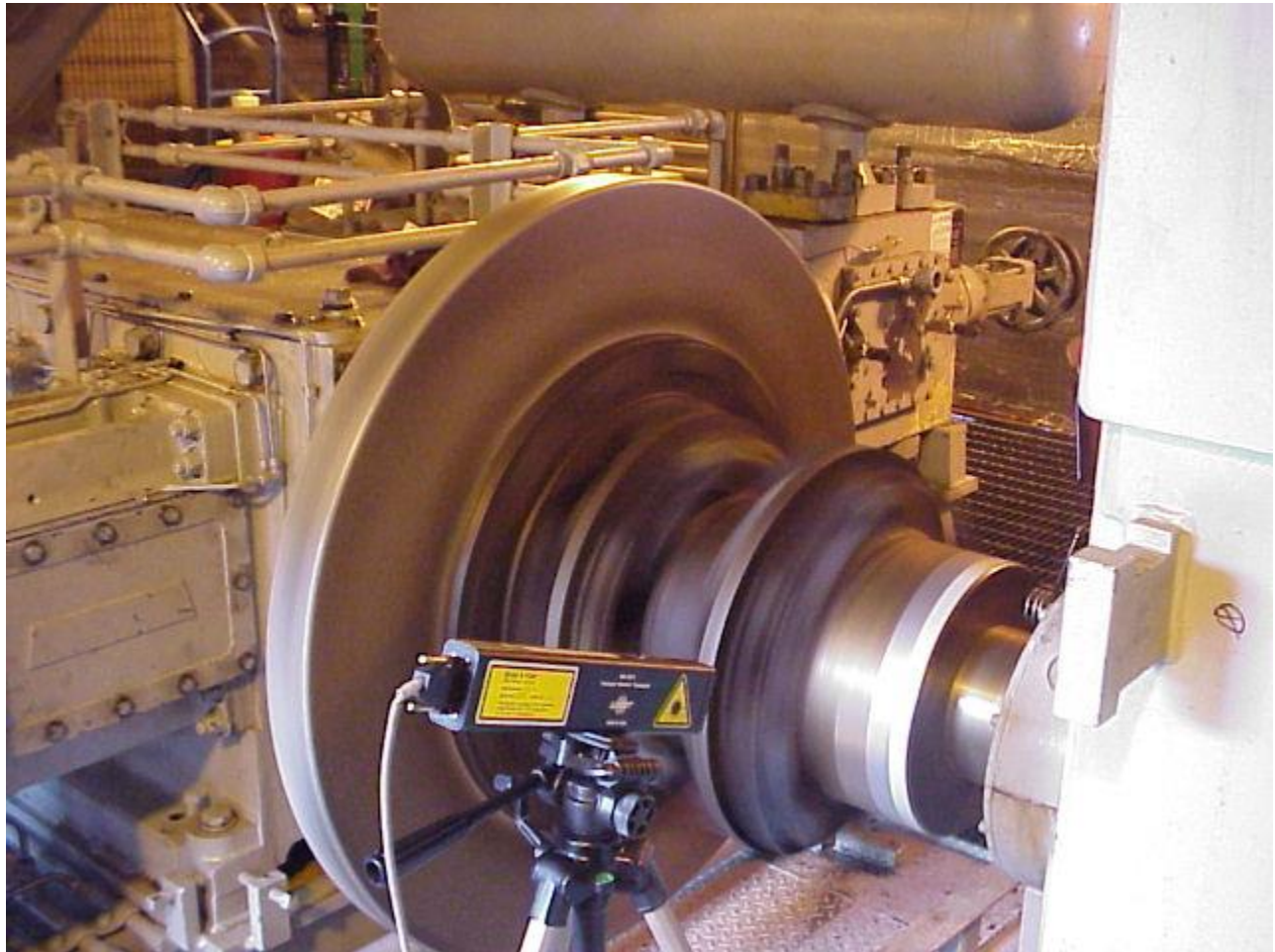
Figure 3.5: Torsional laser vibrometer used to measure torsional vibration at the coupling
