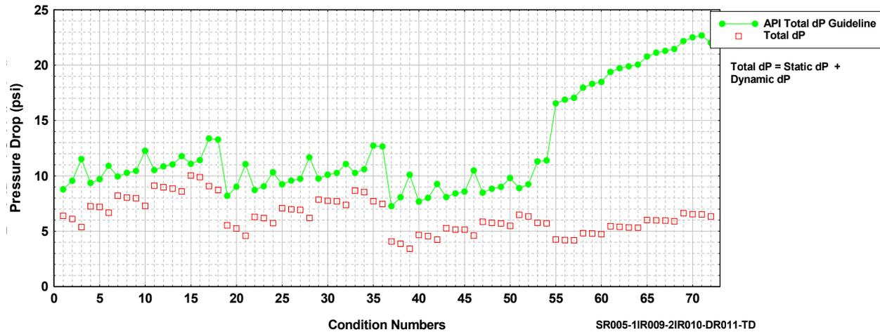
Figure 2.2: Example of Total Pressure Drop Guideline
