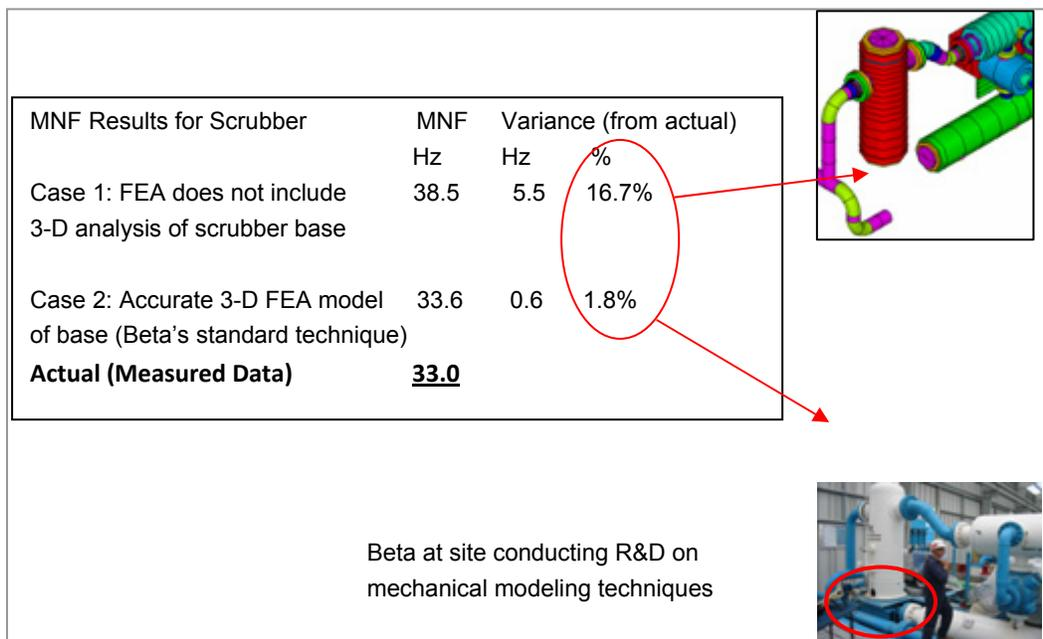
Figure 3.9: FEA Models Must Be Accurate
