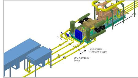
Vibration design studies are routinely performed on compressor packages over 400 HP.
