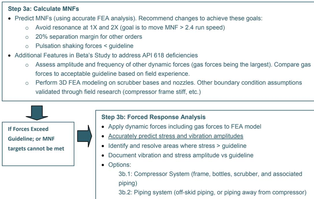
Figure 3.3: Flowchart for DA3 (API 618, 5<sup>th</sup> Ed)
