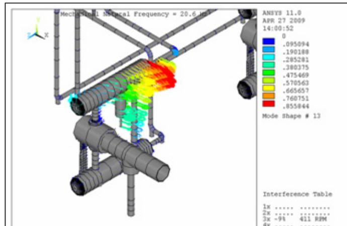
Figure 3.6: Example of 450 RPM Compressor (suction bottles have a MNF of 20.6 Hz. This MNF is -9% below from the 3<sup>rd</sup> order running speed and potentially resonant)
