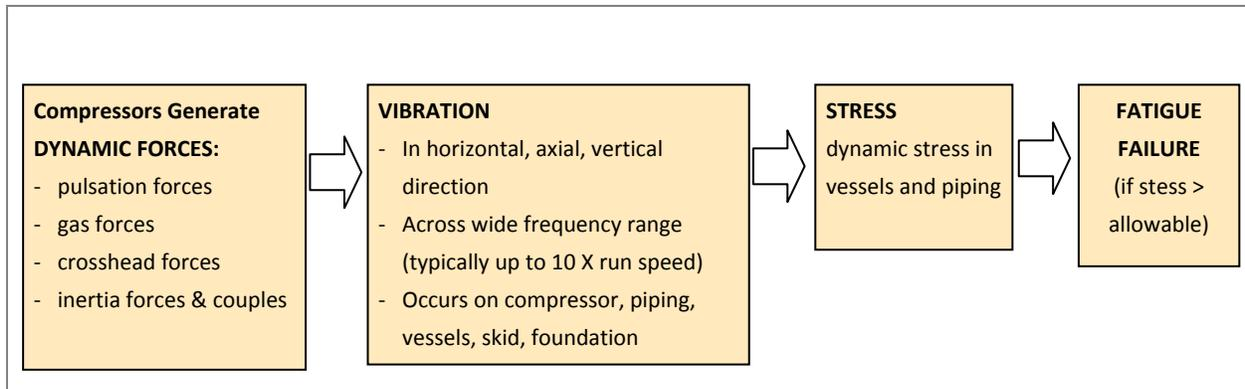
Figure 1.3: Vibration is The Leading Cause of Compressor Downtime (Due to excessive stress on components)
