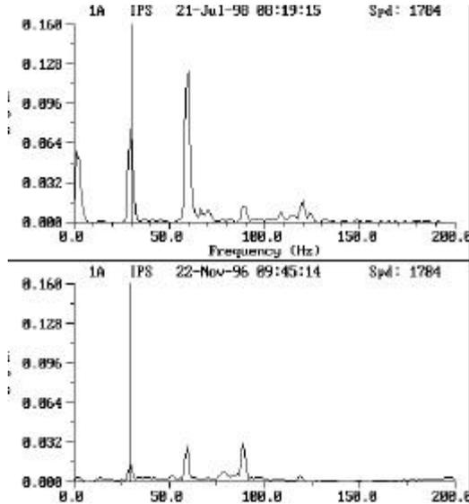
Predictive maintenance programs generally involve analysis of vibration spectra, such as the example to the left. The distinct peaks in the vibration patterns at certain frequencies are due to machine behaviour; the challenge is to determine whether the behaviour is problematic. Notice in this case that there has been a large increase in some components compared to the 22-Nov-96 baseline.
