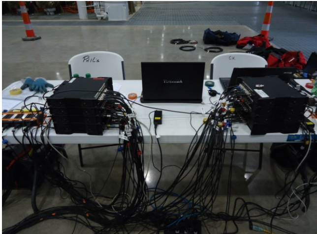
Figure 2: Multi-channel data acquisition system
