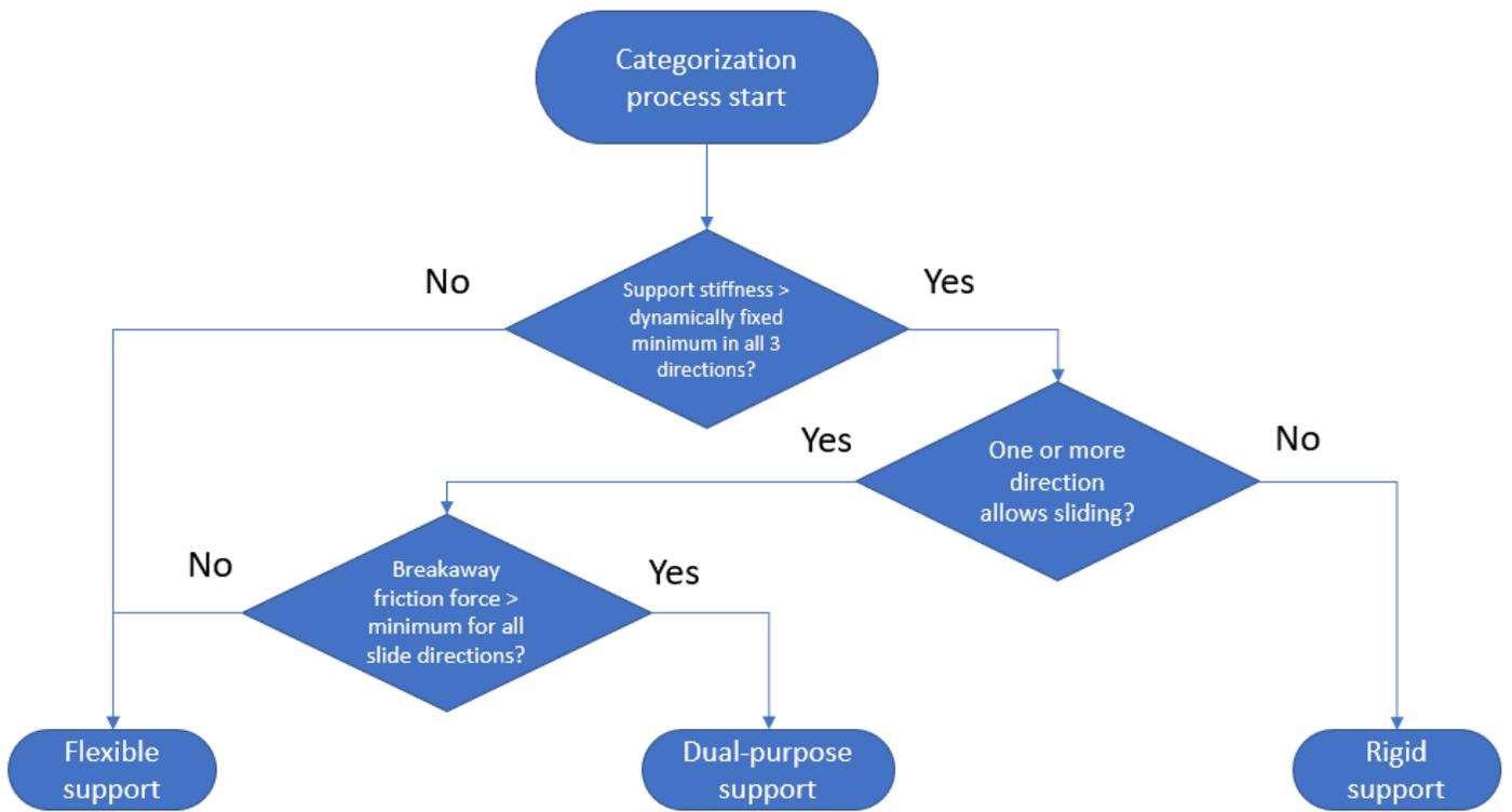
**Figure 9: Pipe support classification flow chart**
