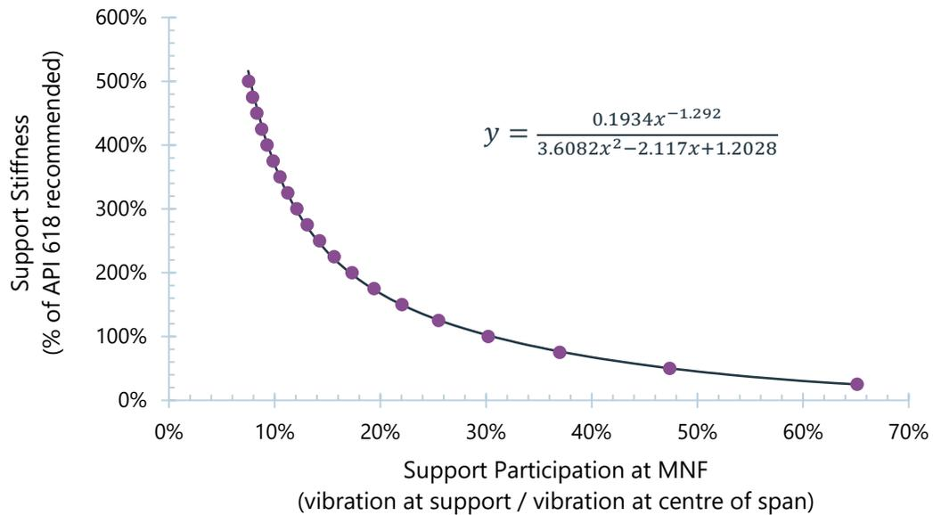
**Figure 13: Relationship between support stiffness and pipe participation for a single span pipe**
