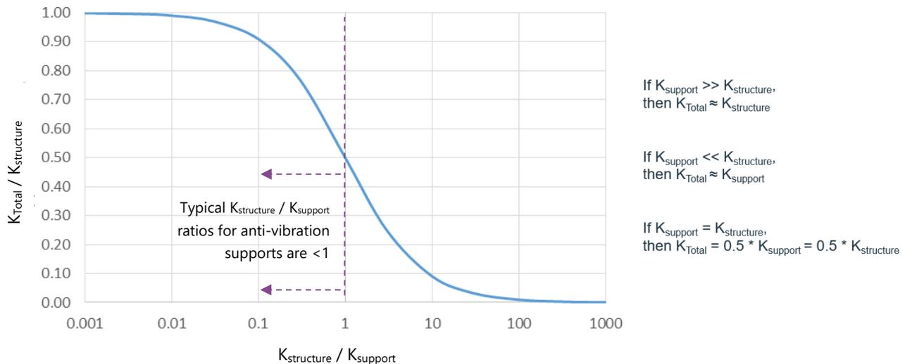
Figure 5: Dependence of total stiffness on the pipe support and structural stiffnesses
