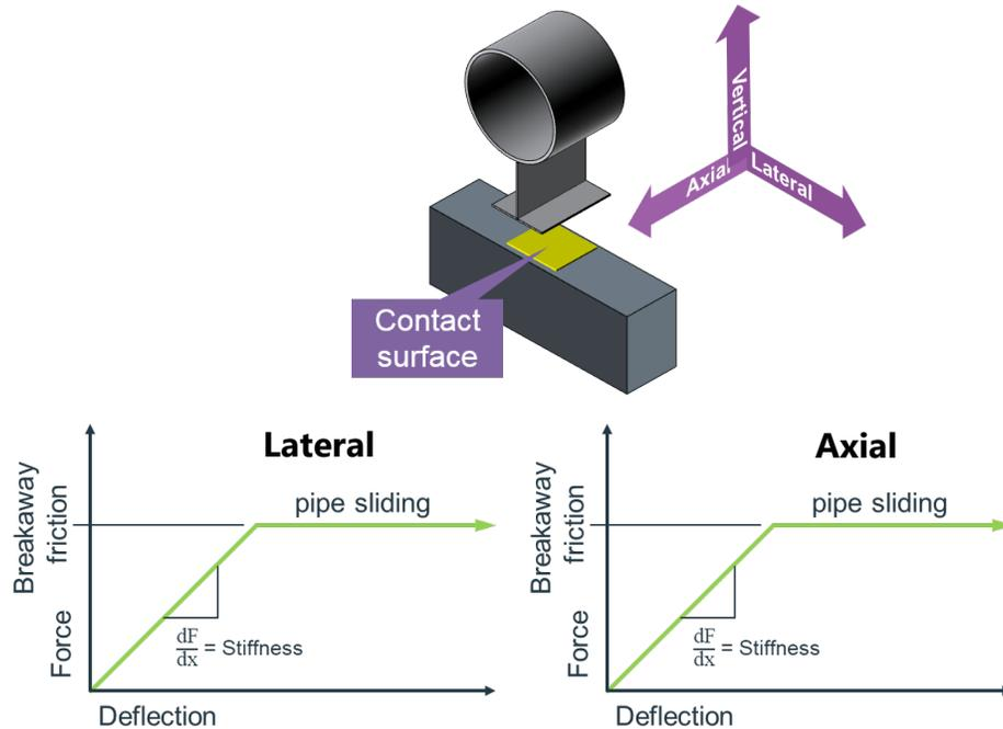
**Figure 6: Sliding support force/deflection relationship per direction**
