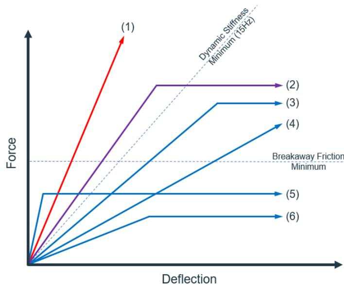
**Figure 10: Force/deflection relationships for various pipe supports**
