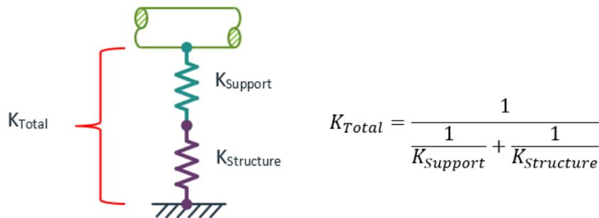
Figure 4: Total stiffness at a pipe support
