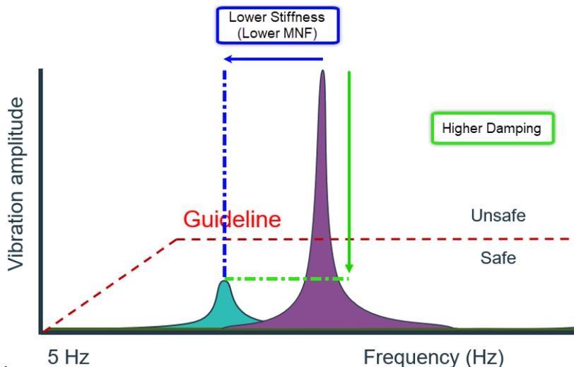
**Figure 8: Typical comparison of a pipe support with and without damping**
