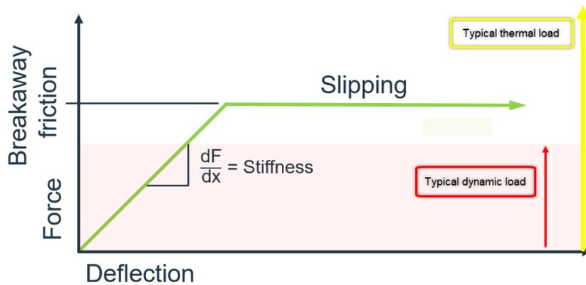
**Figure 7: Typical dynamic and static load magnitudes at a pipe support**
