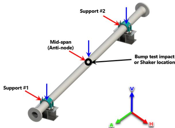
Figure 14: Stiffness measurement setup
