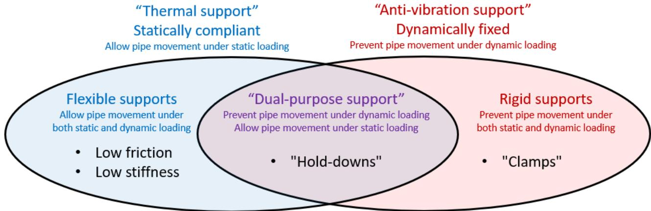
Figure 1: Type of piping supports
