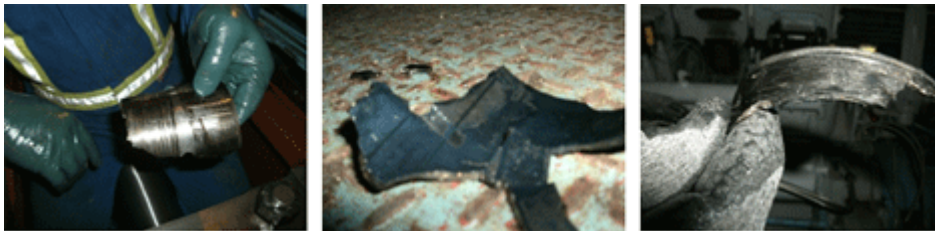
Connecting rod bushing failure
