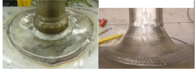
**Figure 8:** Butt weld Pipet with a partial wrap (LEFT) Sweepolet (RIGHT).
