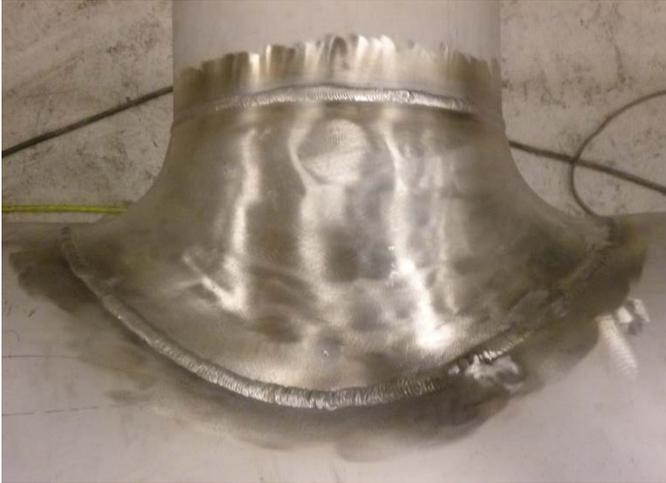
**Figure 5:** Sweepolet tee (NPS 12x20)
