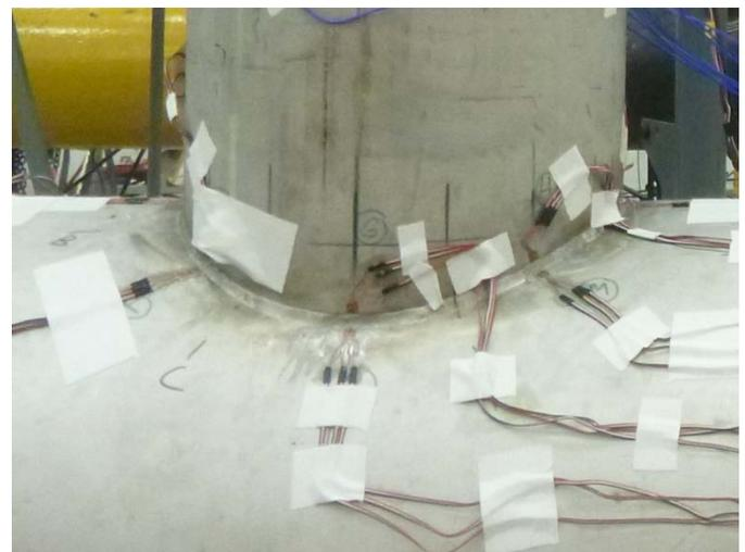
**Figure 3: Stub-on tee (NPS 12x20)**
