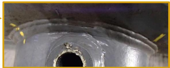
Figure 1: Fatigue crack located between discharge pulsation bottle nozzle reinforcement pad and coupling
