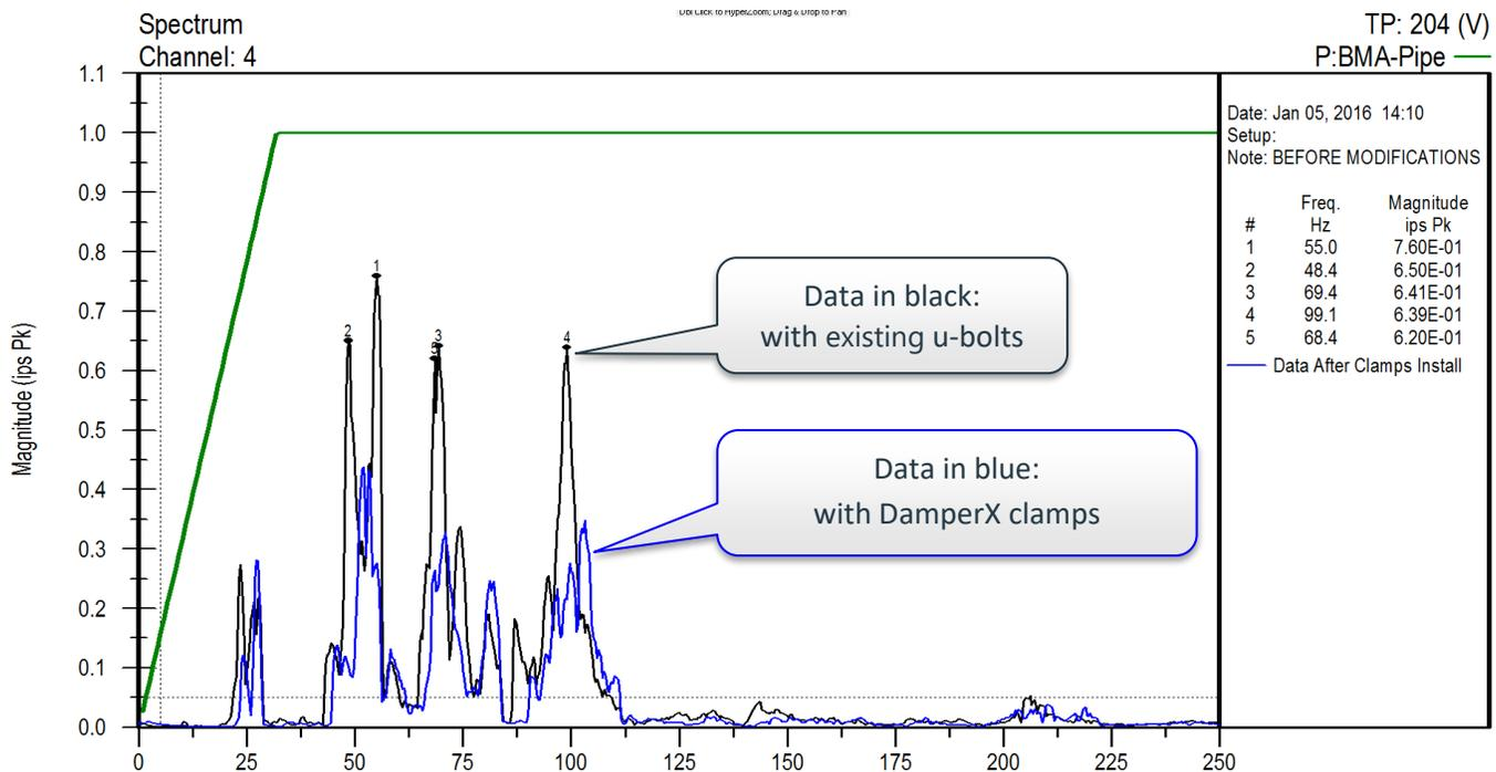
Figure 11 – Operating vibration of main discharge pipe vertical direction (before and after TP #204)
