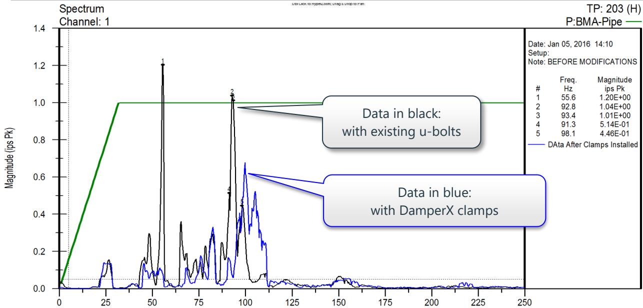
Figure 8 – Operating vibration of main discharge pipe horizontal direction (before and after TP #203)
