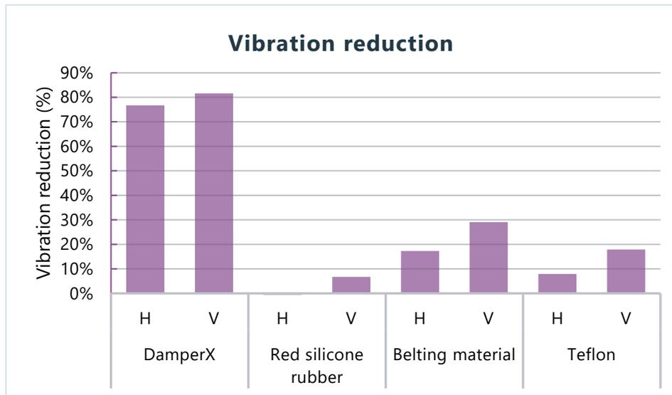
Figure 3 – Vibration reduction by lining, as a percentage of an unlined steel clamp
