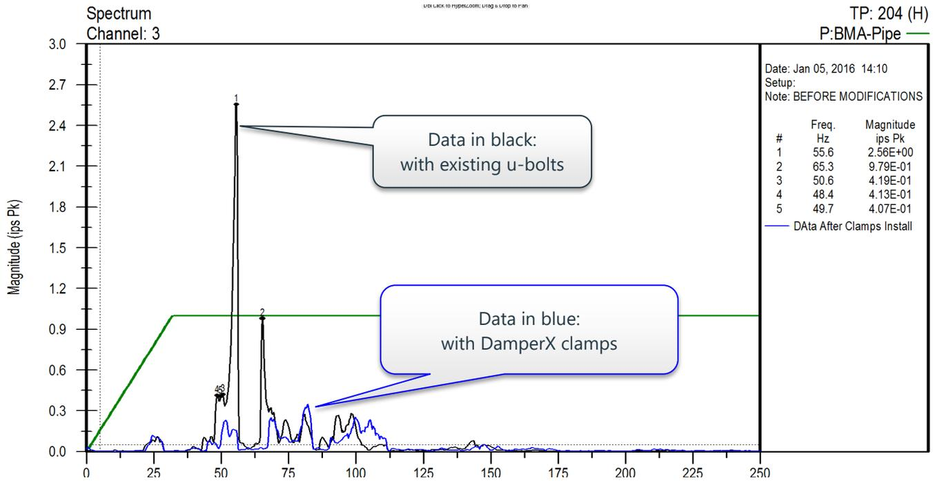
Figure 10 – Operating vibration of main discharge pipe horizontal direction (before and after TP #204)
