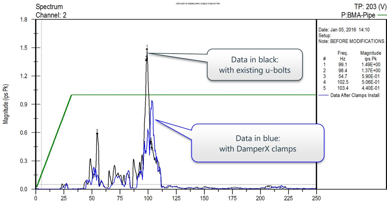
Figure 9 – Operating vibration of main discharge pipe vertical direction (before and after TP #203)
