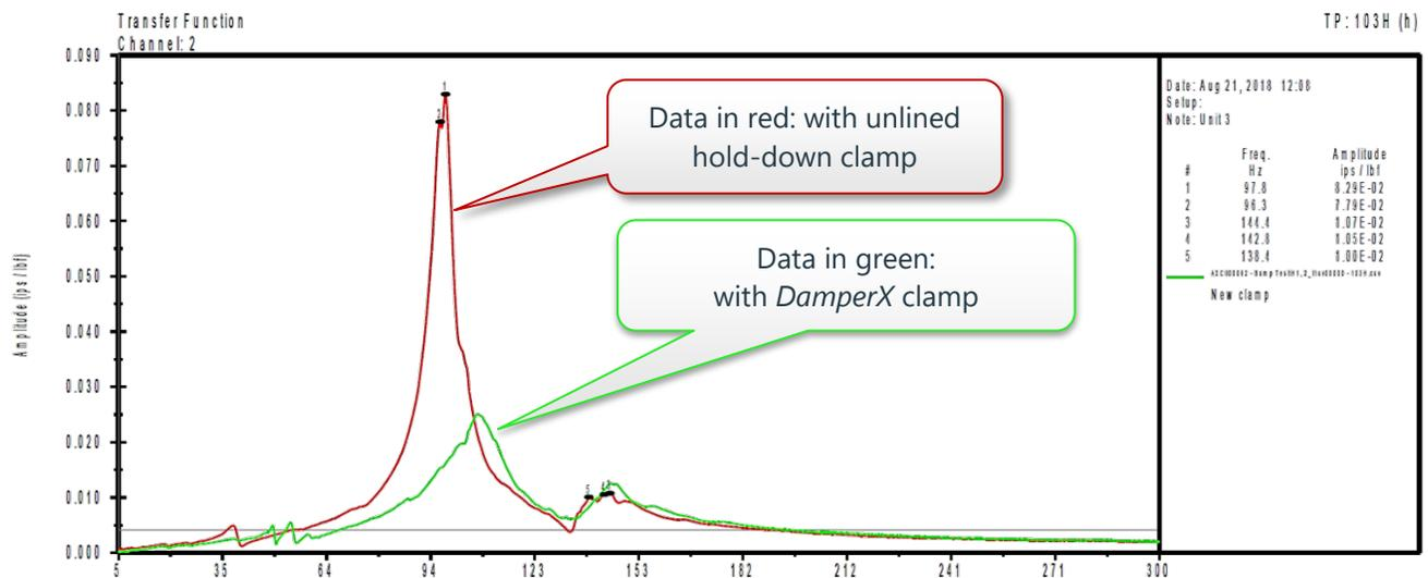
Figure 7 – Impact test of main discharge pipe horizontal direction (before and after TP #103)
