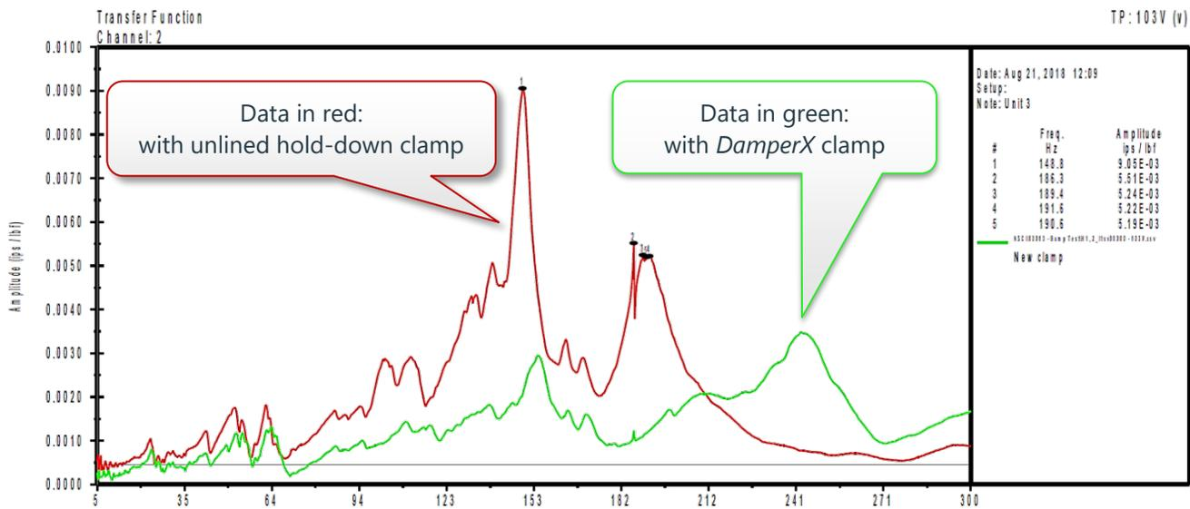
Figure 6 – Impact test of main discharge pipe vertical direction (before and after TP #103)
