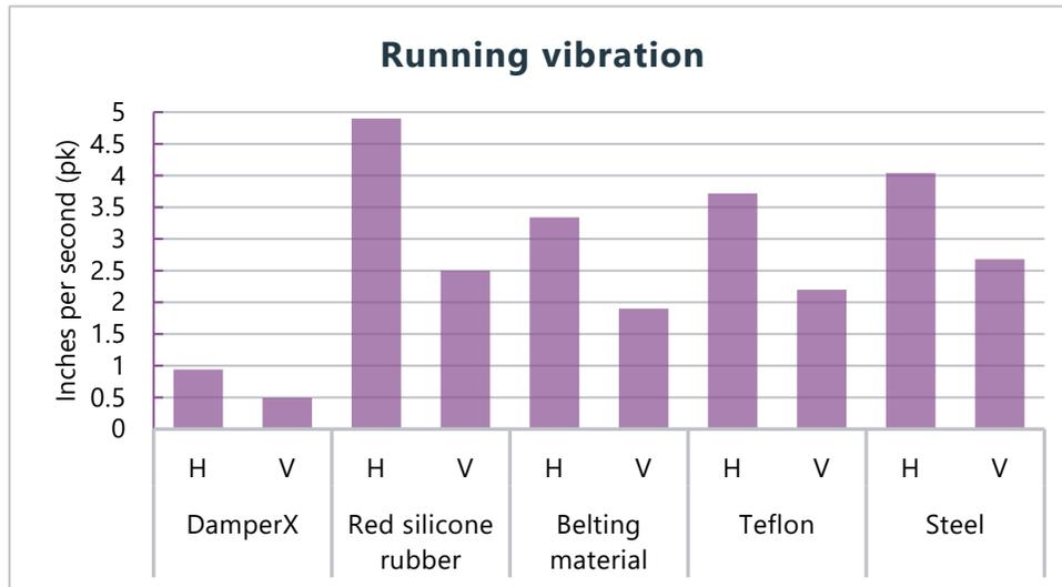
Figure 4 – Running vibration by lining
