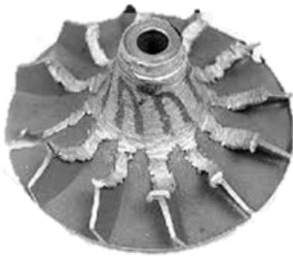
Compressor impeller damaged during surge
